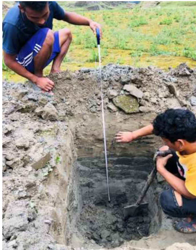
Figure 10: Measurement of old deposition by digging a pit
