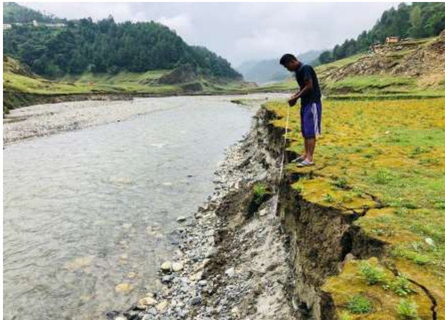
Figure 9: Measurement of deposition from the bed level of river
