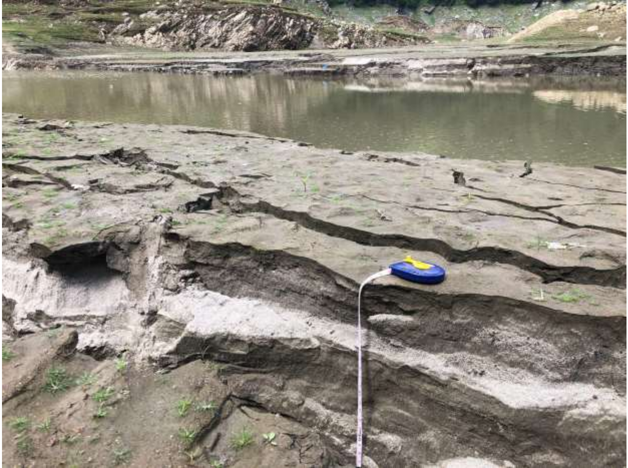
Figure 3: Sand deposit along the banks of Kulekhani reservoir, fissures formed due to undercutting by the water flow
