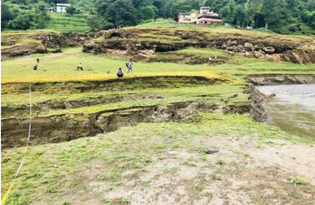
Figure 7: Measurement of deposition on the bank of rivers using tape meter
